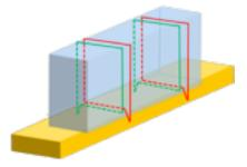
vertikal half loop lashing at not ow case
