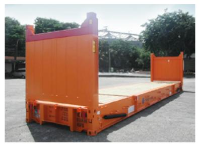
**Welding:** Any kind of welding, drilling holes or modification of a flatrack's structure is strictly forbidden.
