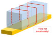
horizontal half-loop lashing against moving to side
