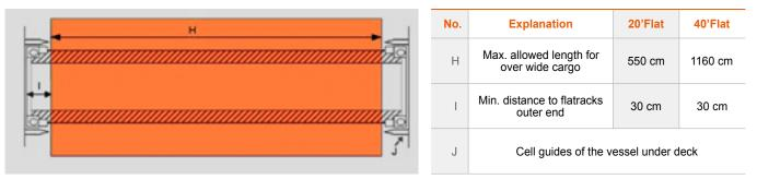
It is important that out-of-gauge measurements are accurate and include the lashing equipment. Incorrect declaration can lead to misrating and short shipment. The width of the floor is less than the container's outer width (244 cms; 96"). Therefore cargo might overlap the flatrack's floor, but still be in-gauge. Only those parts of the cargo or lashing materials which overlap a virtual horizontal line between the outer edges of the corner posts need to be counted as over-width.
