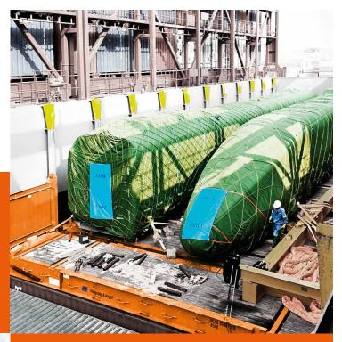
32 metres long: the crane booms that Hapag-Lloyd transported from Rauma in Finland using its own short-sea service via Hamburg, Germany, to Shanghai in China. Belonging to a Finnish firm specialising in mineral extraction equipment, the cranes – together with the driver's cab and accessories that were loaded in separate wooden boxes – weighed over 75 tons. The crane booms were carefully secured on 40' flat racks.
