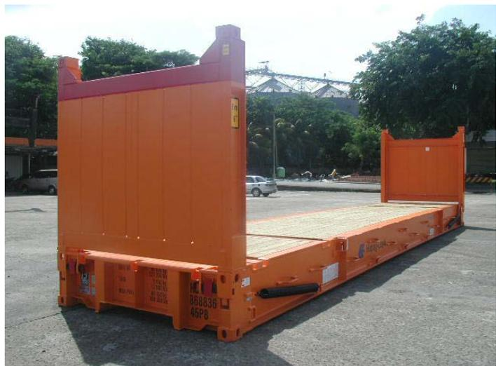
**Bedding.** Any bedding must be laid out across the flat and needs to reach the main girders. Heavy weights are not allowed solely to be place on the wooden floor of the flats. Cargo is to be positioned on the flat with its centre of gravity in the middle of the flat, lengthwise and across.
