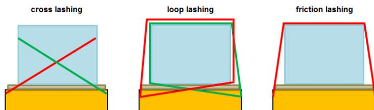
**Lashing calculation.** As a recognised "Rule of Thumb" the number of lashings on each side of the cargo multiplied by the linear or system MSL, must be higher than the weight of cargo. This is valid for optimum lashing system and the number of lashings must be increased when the lashings have bad angles, are bend around narrow radii (wire) or when there are other aspects of less than optimal lashing methods.
