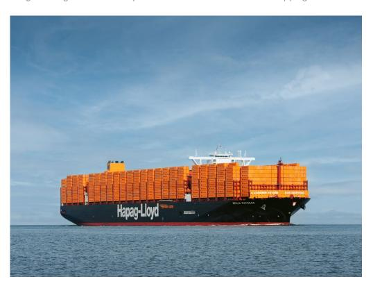
The "Berlin Express" is the first of the new LNG-powered large container ships to enter into service. With a length of almost 400 meters and a capacity of 23,664 TEU, it is the largest container ship to ever sail under the German flag. German First Lady Elke Büdenbender performs the christening ceremony in Hamburg at the beginning of October. The newbuildings and other measures help to steadily improve the fleet's carbon footprint.
