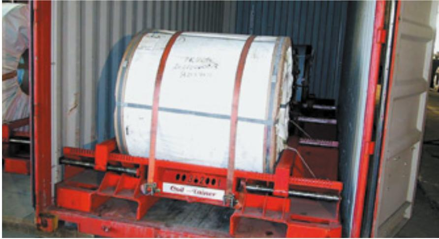
**Steel coil secured on a Coil-Tainer cradle**
