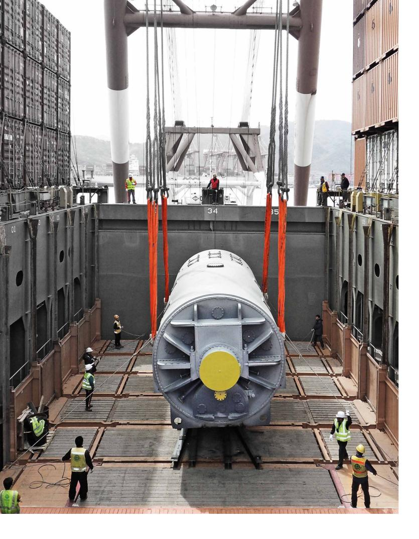
343-ton turbines, 32-metre-long crane booms, 14-metre-wide catamarans - for over five decades, Hapag-Lloyd has been transporting special cargo that does not fit in a standard container.
