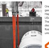
One particularly heavy load was a gas turbine weighing 343 tons that Hapag-Lloyd shipped from Charleston USA, to Busan in South Korea. The heavy cargo was lifted aboard and discharged by the use of contracted floating cranes at the loading port - and unloaded again at the destination port.
